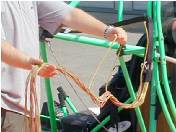
9. Open the throttle continuously at a rate that when the lines are fully straightened the throttle is fully open. And let the canopy climb above your head.
