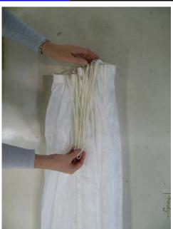
**Apex placement**Place all the apex lines on top of the gores.
