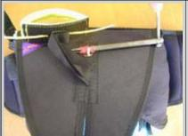
Push a bullet needle through the closing loop and use it to lead the locking cable on the handle through the closing loop.
