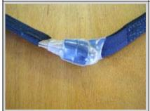
Pass the heat shrink tube over the knot and carefully heat it with a heat gun or hair drier to fix it in place.
