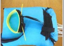
Thread the first (withouth the Split Ring) attachment loop through one of the attachment points on the deployment bag.
