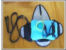
Flip the reserve over onto the central part of the container, making sure the bridle and lines are neatly placed, to avoid the danger of a bag lock.
