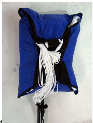
15) Open the knot in the riser bridge, fold it in an "s" shape and wrap it with a rubber band according to Fig.35.
