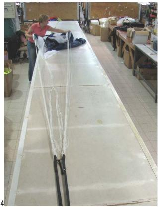
3) Arrange the centre of the parachute so that the centre row of lines lies on top of each other (in order C17, C15, C13, C11, C9, C7, C5,C3, C1)(fig) and fold the right canopy side (In direction of flight) to the left side (fig.6).
