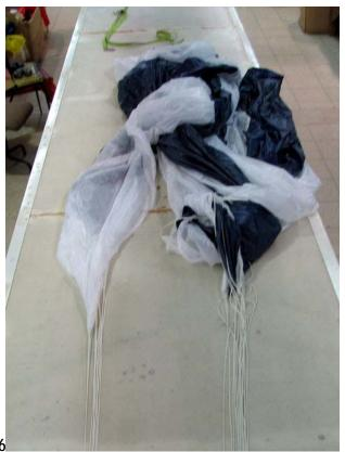
**Note**: Fold the canopy from the trailing edge towards the tip, left and right side separately. Take care that lines are tensioned at all times during packing (pull from the marking dots shown in fig .8 to tension the lines).
