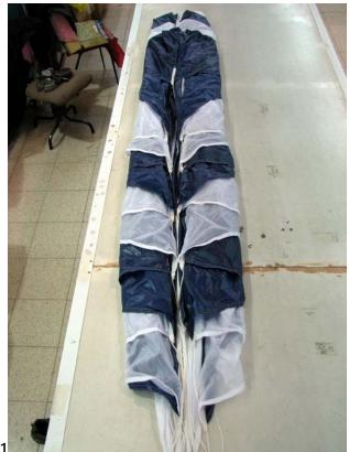
11) Clip one side with padded clips, fold it on the other side, Weigh down the parachute with weights and unclip it according to Fig.22-23.
