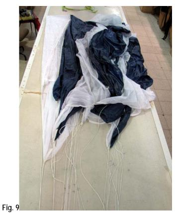
Arrange the other sections so that the tape from the support line lies immediately next to and parallel to the arranged parachute centre. The bottom edge of the section is folded towards the parachute centre (Fig. 9)
