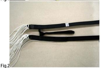
Divide the lines into a right and left half. The border between the left and right section in the canopy is a 2,5 cm thick riser with central lines. With the parachute arranged in this manner, lay it on the packing table with the trailing edge towards the ground and tip pointing upwards. Check that lines pass freely from the "H" riser to the canopy in the following order: Br, C17, 15, C15, 13, C13, 11, C11, 9, C9, 7, C7, 5, C5, 3, C3, C1(fig.3).
