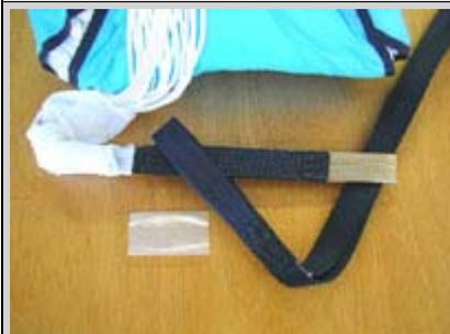
Pass the two free ends of the V-Bridle through the loop in the reserve bridle.
