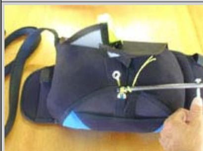
Use a rigger's wrench to pull the closing loop through the grommets and use a bullet needle to lead the second locking cable from the deployment handle through the closing loop.
