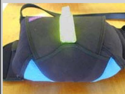
Pull the neoprene pocket on flap No.4 up towards the deployment handle by the two velcro strips in its center. Tuck the two velcro strips under the handle and press the handle down to fix it in place.
